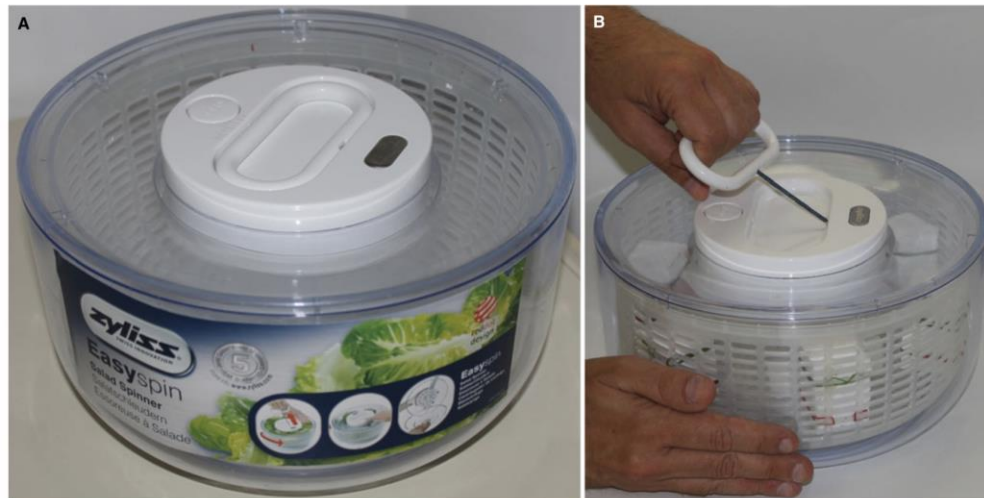
Figure 1. Manual cytocentrifugation method using a modified commercially available salad spinner (A), with a cord attached to a handle (B).
